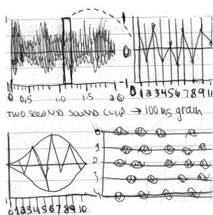
**Figure 12.** An early sketch from one of my notebooks about how to granulate sound files in real time. The sound file is converted into a simplified 8-bit version, and a grain (shown lower-left) is shown operating over several streams.
