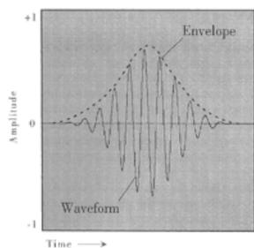
**Figure 5.** A visual depiction of an audio grain, shaped by a Hanning Function. The contents of this grain are sinusoidal in nature.
